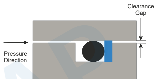
With backup ring Blocks extrusion and supports the O-ring
